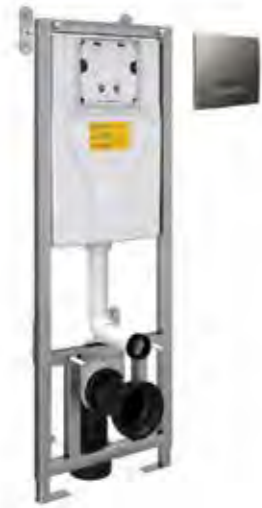
WC Frame & Cistern With Chrome Flush Plate 3 and 6 litre flushing option, adjustable height, weight limit 400kg, silent filling and 3-7 bar operating pressure
